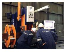
multipurpose and can be configured to allow the machine to cut pipes and box sections (ranging from 48mm diameter to 610mm diameter piping and 60mm x 60mm SHS to 450mm x 450mm SHS). The advantages it offers has further increased Belmet's workflow efficiencies.
