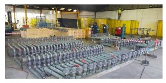
required 3C Metal South Africa to establish production lines with customized jigs for the fit-up and welding of the piping spools.
