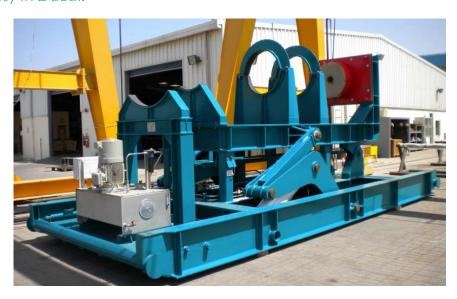
and foolproof system incorporating several safety and interlocking methods. ATH & Veraflex supplied the cylinders as well as the HPU's for all of the Skids from France.
