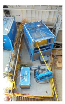
The upgrade involves the integration of structures, piping, sheave attachment points and electrical connections for various well completion systems including the Intervention Workover Control System (IWOCS) from OneSubsea and the Halliburton Subsea Safety System (TSS) for the Upper Completion.
