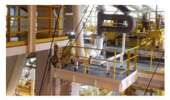
3C Metal was requested to follow the same integration route, where the Coriolis loop runs as a bypass of the rig's main flowline and is located beneath the drill floor near the diverter. 3C Metal provided a system on which all knife valves are pneumatically actuated and controlled by a pneumatic panel located on the drill floor. The panel contains an interlock that prevents the bypass valve from being closed when the valves on the loop are shut - mitigating the possibility of accidentally
