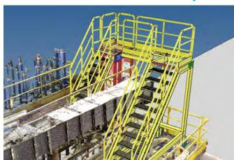
The client requested an efficient and safe access solution from the rig's starboard jackcase to the cantilever to minimize the route for onboard personnel. This request aimed to improve operational efficiency and ensure safety for the crew.
